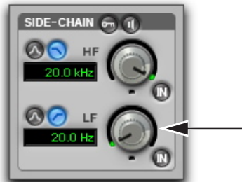
LF frequency controls
