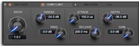
Dynamics section, Compressor/Limiter tab
